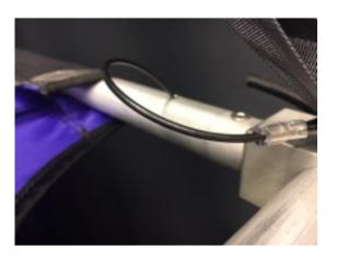
6. Go to the other side and repeat. This side will be easier as the other end is holding the ledge open. Go back to the other side and make sure it is 100% locked in. Trying to push the ledge into a rhombus shape helps. Smack the corners with the palm of your hand. They all should click in.
